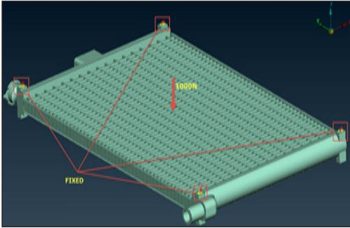
Figure 3. Analytical model for first boundary condition (Load Case 1)
