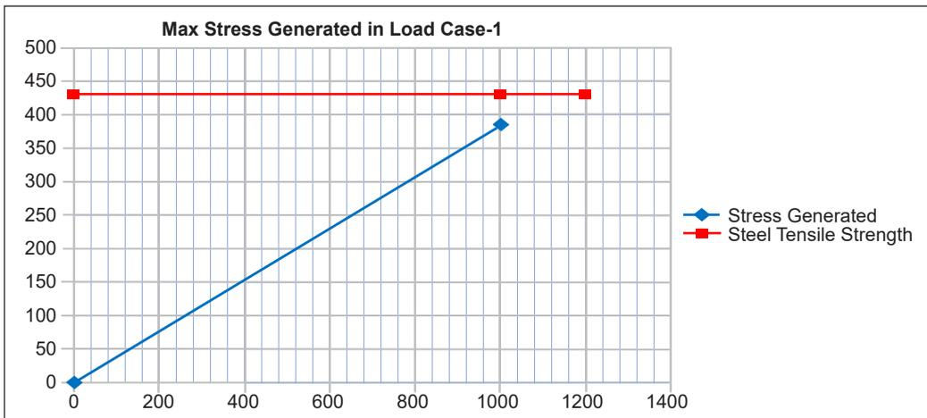
Figure 13. Steel maximum stress generated load case 1
