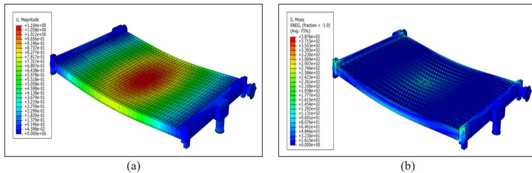
Figure 5. (a) Deflection and (b) stress distribution plot for steel in load case 1
