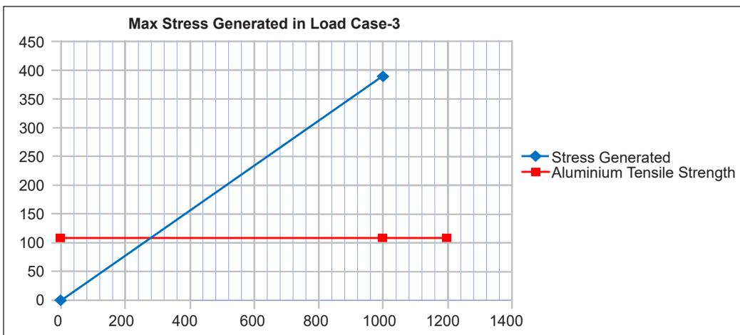
Figure 14. Aluminium maximum stress generated load case 3
